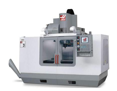
Super-Speed Vertical Machining Center; 50" x 26" x 25" (1270 x 660 x 635 mm), 40 taper, 30-hp (22.4 kW) vector drive, 12,000 rpm, inline direct-drive, high-speed 24+1 side-mount tool changer, 1200 ipm (30.5 m/min) rapids, power-failure detection module, 1 GB program memory, 15" color LCD monitor, USB port, memory lock keyswitch, rigid tapping and 95-gallon (360 liter) flood coolant system.
